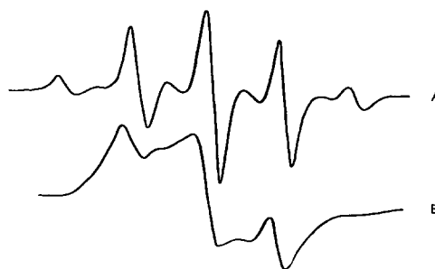
Figure 11 Change in the e.s.r. spectra from A, 50 wt% EGDMA, polymerized for 100 min, to B, reacted with the swelled styrene monomer for 10 h thereafter. Gain: A, 5 \times 10^4 ; B, 5 \times 10^5 . Other e.s.r. conditions as in Figure 7. T = 70^\circ\text{C} ; AIBN, 0.3 wt%
